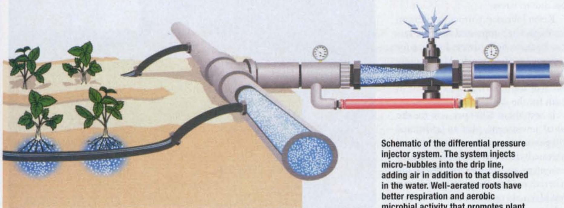
Schematic of the differential pressure injector system. The system injects micro-bubbles into the drip line, adding air in addition to that dissolved in the water. Well-aerated roots have better respiration and aerobic microbial activity that promotes plant health.
