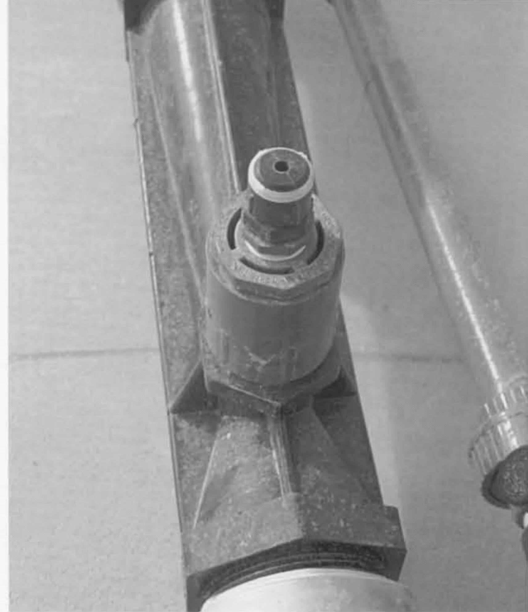
The part of the Mazzei system that sucks in air and sends it into the distribution line.
