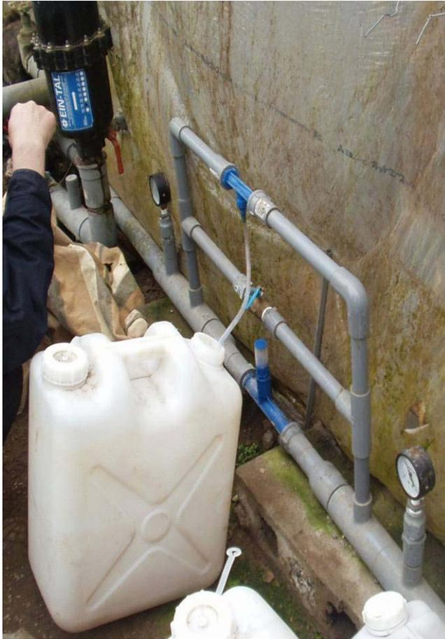
The lower Mazzei injector worked with sucking Air, and upper Mazzei injector sucked fertilizer. The middle valve controls separation of water flow. Fertilizer can be more controlled with the attached liquid flow gauge. Left side upper are pre 200-mesh filter. Both side gauges show pressures. The white tank is a liquid fertilizer.
