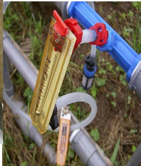
The Fertilizer mixing unit usually works each time of irrigation. The cylinder was connected by a soft-tube with the sucking fertilizer unit. About 0.3mm stainless-steel mesh is installed in order to avoid the risk of foreign articles to be sucked.
