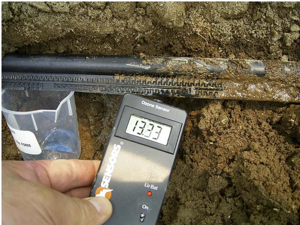
Upper photo shows the direct detection from a out-let, which emits bubbles with ozone, of irrigation tube. For your reference, we take off the sensor cover for this photo. The water sample was collected in the plastic beaker and analyzed through coloring reagent. Measure tool showed good evidence that this Ozone-gas-injection-system was supplied through gas-phase methods.
