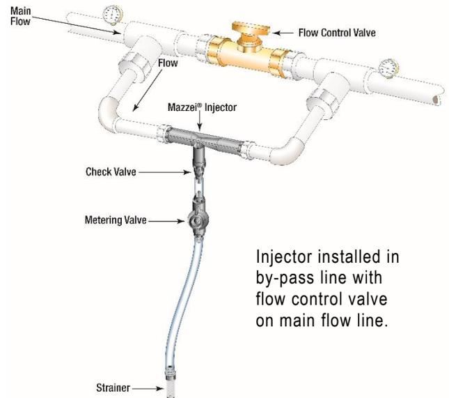
Injector installed in by-pass line with flow control valve on main flow line.
