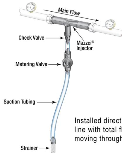
Installed directly in the main flow line with total flow of the system moving through the injector.
