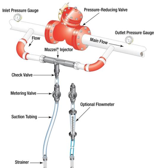
Injector installed around a point of restriction, such as a regulator valve or gate valve, which creates a differential pressure, thereby allowing the injector to produce a vacuum.
