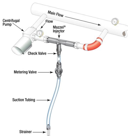
Installed in conjunction with a centrifugal pump to boost pressure through the injector thereby creating a differential pressure and producing a vacuum for chemical induction downstream from the pump.
