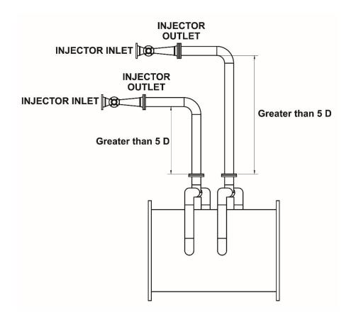
D = Nominal Pipe Size of Injector Inlet/Outlet Connection
