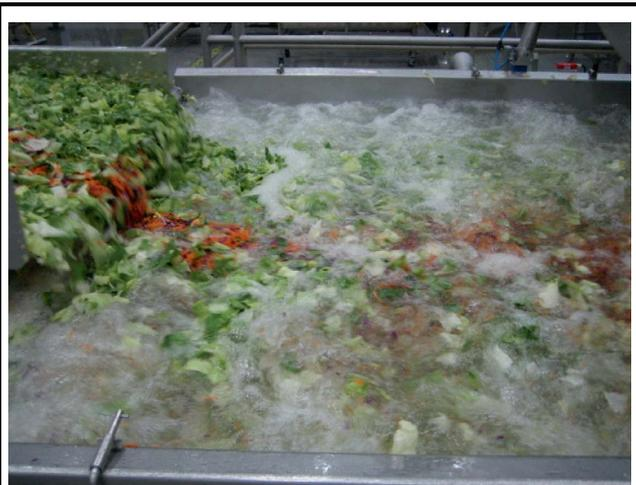
**FIGURE 6.** Food Technology Noord-Oost Nederland B.V. – Because the FTNON unit provides a large amount of agitation, ozone off-gassing was measured in and around the unit utilizing an Aeroqual Series 300 ozone monitor (Photo supplied by Noord-Oost).
