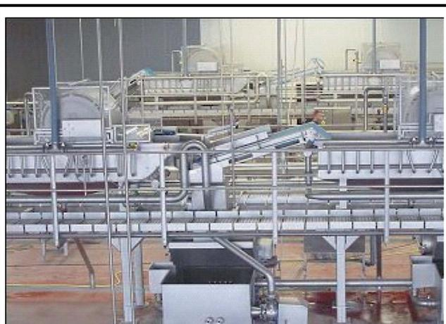
**FIGURE 1.** Food Technology Noord-Oost Nederland B.V. (FTNON) is a specially developed flotation washing machine for washing products such as fruits, (leaf) vegetables, mushrooms etc. (Photo supplied by Noord-Oost).
