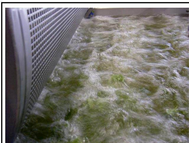
**FIGURE 3.** Food Technology Noord-Oost Nederland B.V. — As product moves through the FTNON unit, agitation removes non-vegetative materials. Heavier particles such as sand and mineral particles settle and light particles such as insects and insect fragments flow through the rotating drum and are removed in a side stream (Photo supplied by Noord-Oost).
