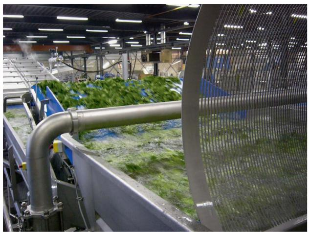
**FIGURE 4.** Food Technology Noord-Oost Nederland B.V. – After product moves under the rotating drum, it is conveyed to a second unit and washed again. Water temperatures are maintained and chlorine levels are checked frequently (Photo supplied by Noord-Oost).
