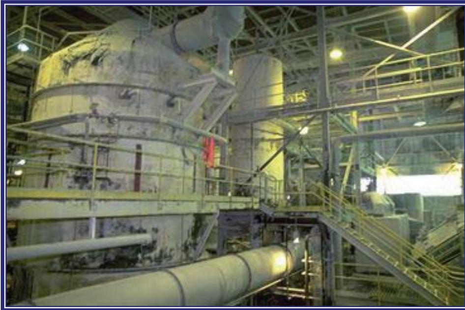
**Figure 2.** Evaporator for sodium carbonate monohydrate crystal growth, courtesy OCI.
