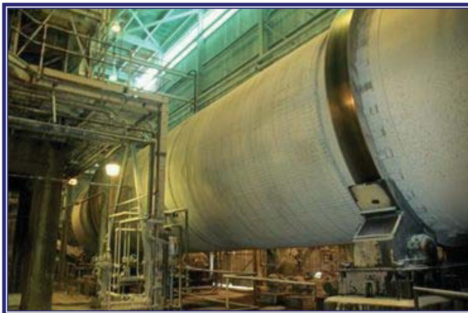
**Figure 1.** Kiln heating of crushed Trona ore courtesy OCI Chemical Corporation.
