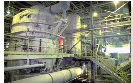
**FIGURE 1:** Evaporator for sodium carbonate monohydrate crystal growth
