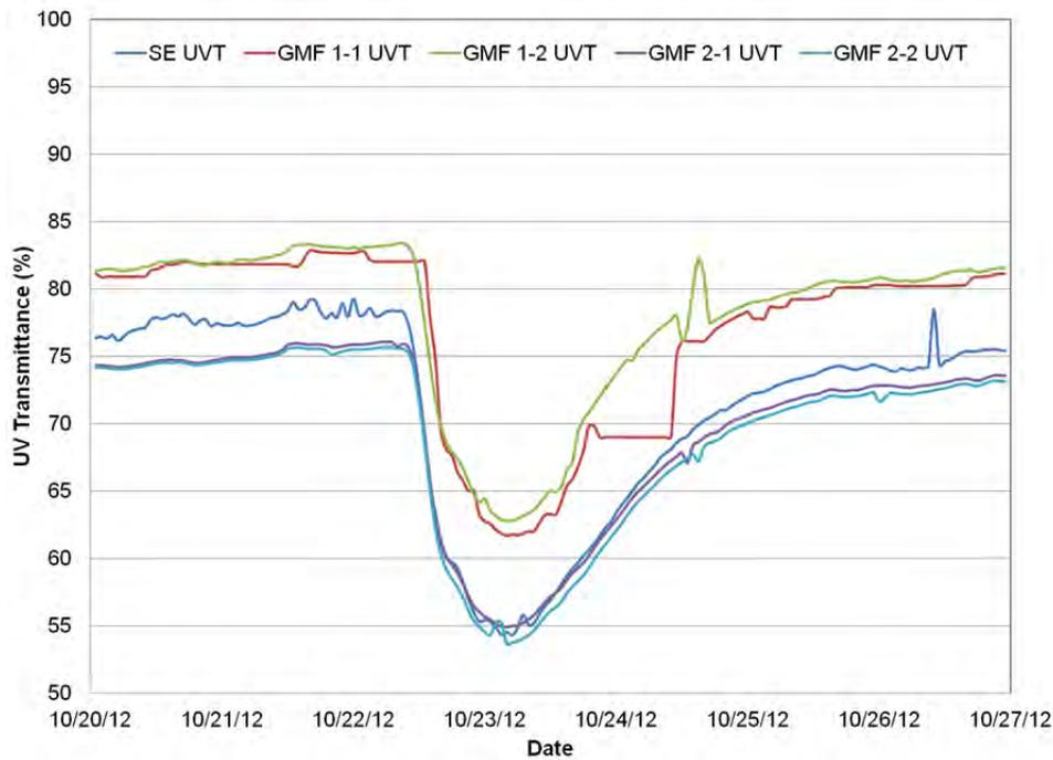
Figure 9. Effect of ozone on UV Transmittance
