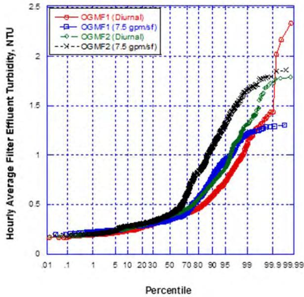
Figure 4. Probability plot of CGMF effluent hourly average turbidity data.
