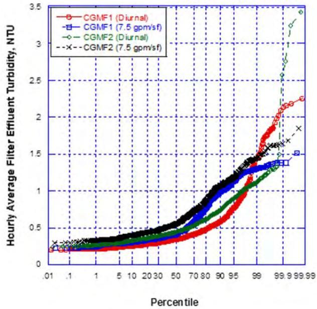
The Title 22 turbidity limit for membrane filters is 0.2 NTU. The data presented in Figure 5 illustrate that the test MF system met the Title 22 turbidity requirements.
