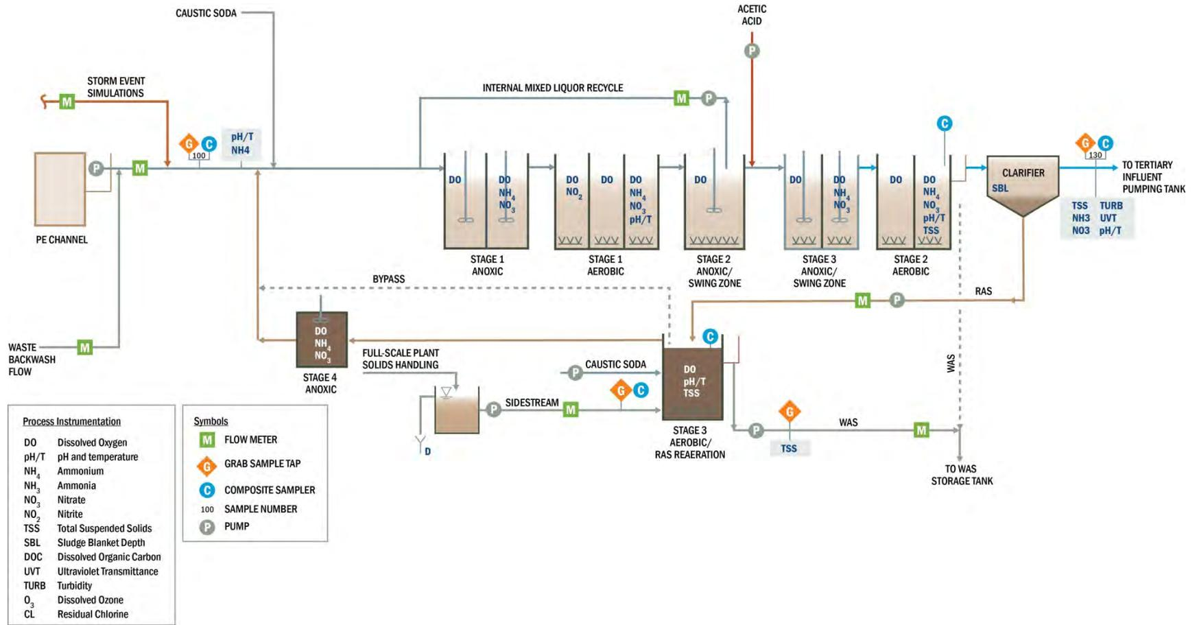
Figure 1. SRWTP Advanced Treatment Technology Pilot Project Tertiary Treatment TOC Sample Locations
