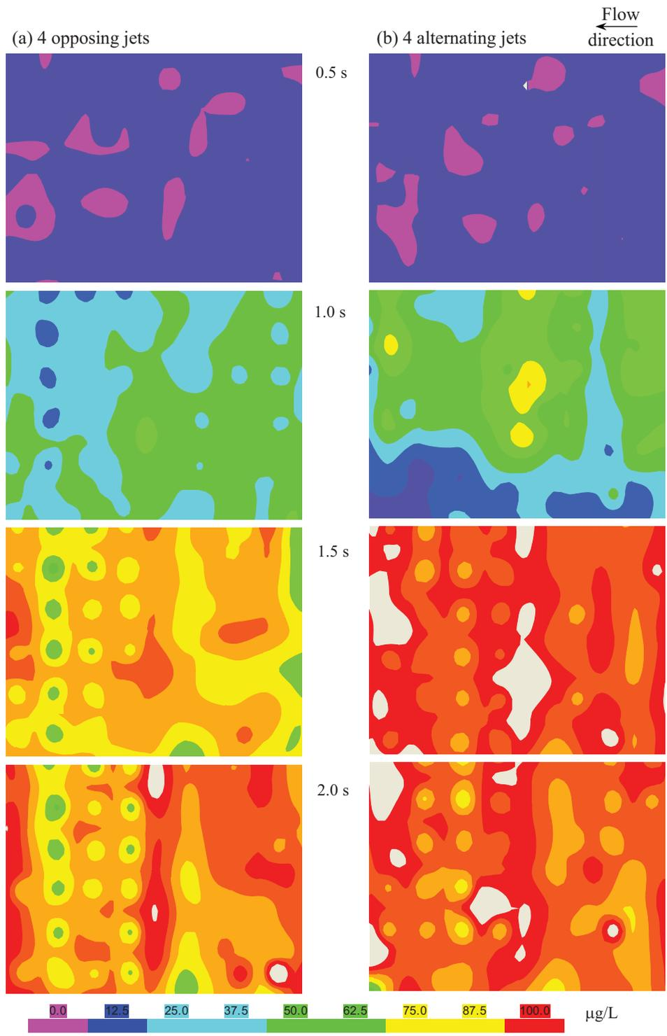
**Figure 2.** Tracer concentration for 4 jets (opposing and alternating).
