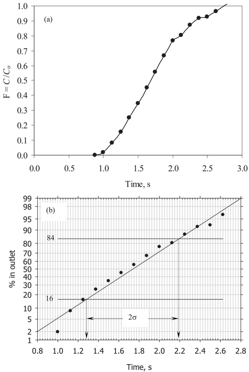
**Figure 4.** Step response curve and probability plot of the response signal for 4 alternating jets [adopted from Baawain et al. (2007)].
