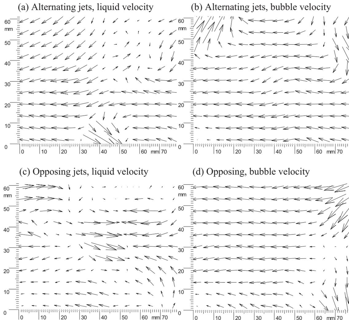
**Figure 3.** Velocity vectors for alternating and opposing jets at inlet zone (scale: 5 mm = 1 m/s) [adopted from Baawain et al. (2007)].
