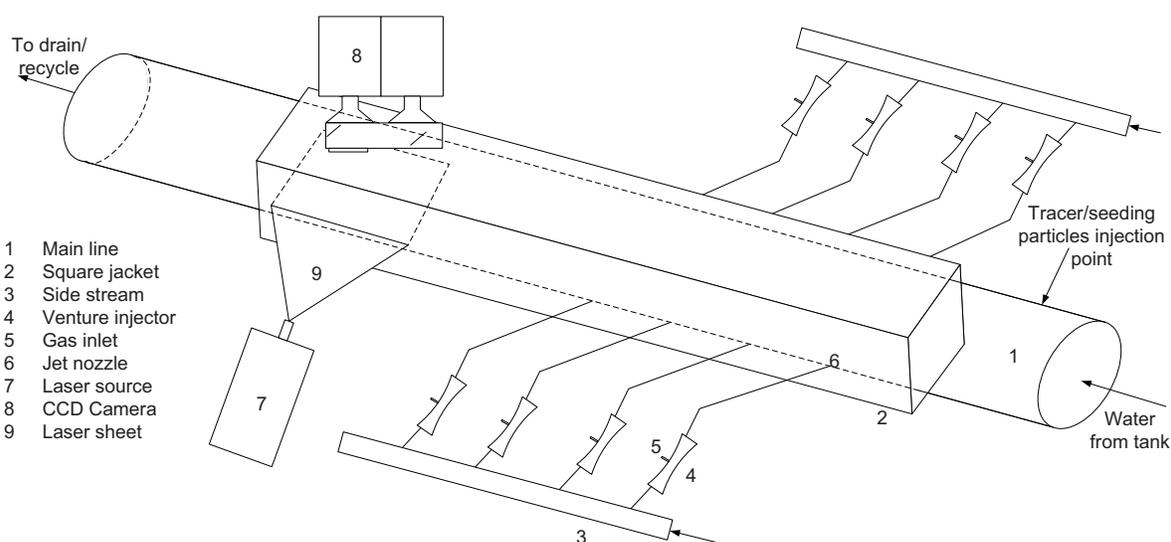
**Figure 1.** Experimental setup [adopted from Baawain et al. (2007)].
