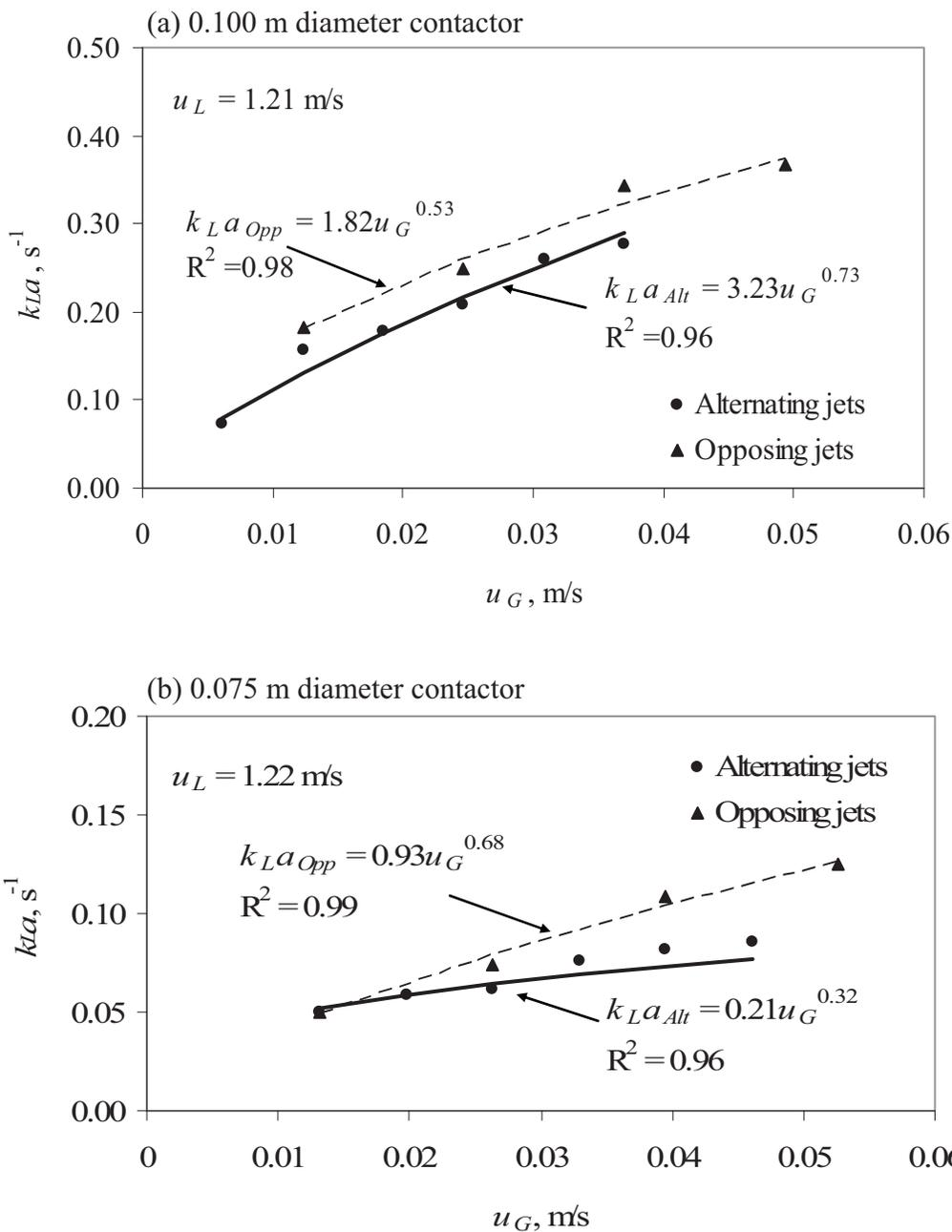
**Figure 5.** Overall mass transfer rate for alternating and opposing jets for the two ozone contactors.
